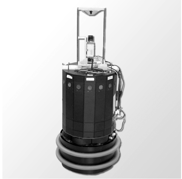
Figure 1: Omnidirectional camera mounted on the top of the Nomad 200 mobile robot.
