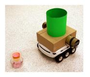
**Fig. 1.** Koala Robot with the Örebro Mark III mobile nose.
