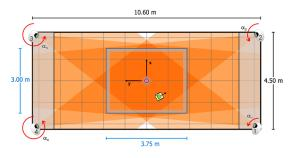
Fig. 2. Floor plan of the used laboratory room together with an outline of the area inspected.
