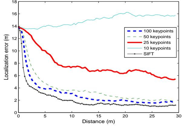
**Fig. 7.** Localization error against distance travelled by the robot using different number of keypoints.  $NTrials = 7$  in all the experiments.
