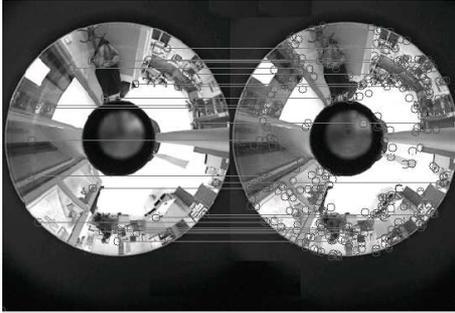
**Fig. 6.** Matching two different panoramic images using the proposed approach. Only a small number of features are required to get the same matching image.
