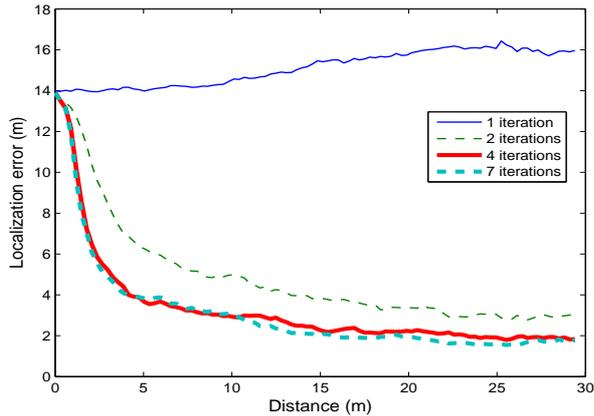
**Fig. 8.** Localization error against distance travelled by the robot using 100 keypoints and different number of iterations ( $N_{trials}$ ).
