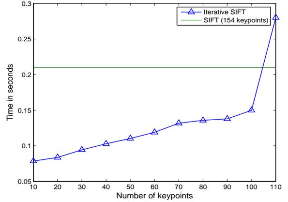
**Fig. 3.** The time required to extract a given number of keypoints on a sample images, including the time of calculating the DoG, done with a 3GHz Pentium.
