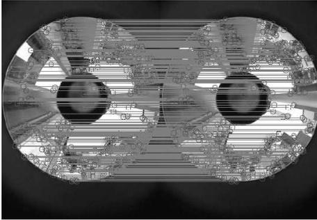
**Fig. 2.** Matching two different panoramic images using SIFT. The number of common features is huge, requiring a high computation time.
