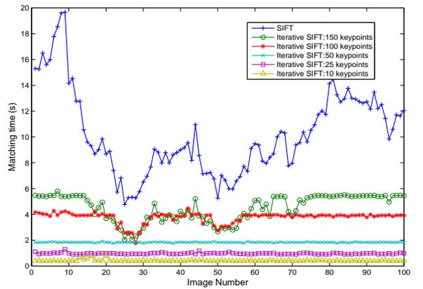
**Fig. 4.** The time required to extract and match a given number of keypoints using iterative SIFT versus the time of SIFT for a set of 100 images, done with a 3GHz Pentium.
