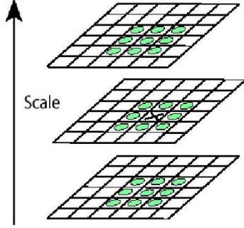
**Fig. 1.** Local extrema detection. The pixel marked  $\times$  is compared against its 26 neighbours in a  $3 \times 3 \times 3$  neighbourhood that spans adjacent DoG images (from [6]).
