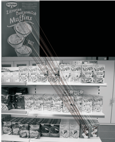
Figure 4 Vision-based product recognition. The package shown in the upper part of the figure is contained in the database. The lower part of the figure shows the current view of the robot, in which the product is detected twice.
