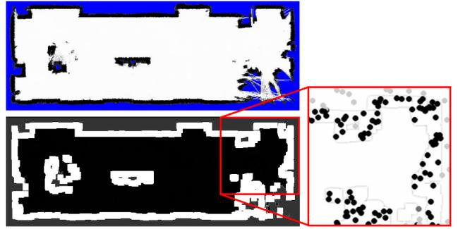
Fig. 4. Illustration of our structural initialization approach. *Upper left*: The occupancy grid representing spatial structure. *Lower left*: Contour detection for the optional case that tags are expected to lie on the outer side of objects. *Right*: Close-up of the map, showing a random initial assignment of particles to occupied cells. Particles are represented by the small circles, where darkness corresponds to weights.
