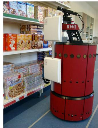
Fig. 1. The mobile platform (RWI B21) with on-board UHF RFID reader, RFID antennas (white), and laser scanner (behind lower antenna) for self-localization. Passive RFID tags were used that were attached to the product packages in the shelf as well as to furniture and walls.
