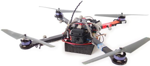
**Figure 1:** Tests were done on an AscTec Hummingbird quadcopter.
