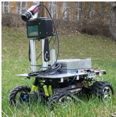
Figure 4: Robot with mounted 3D laser ranging sensor
