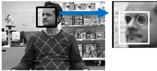
Fig. 3. Example of eye tracking and face cropping. White circles indicate locations of the eyes. The white rectangle indicates the location of the cropped face.
