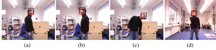
Fig. 2. Examples of face tracking through occlusion and drift. We compare our face tracker, which is marked by the red rectangle, and the original MOSSE filter, which is marked by the black rectangle. 2(a), 2(b), 2(c): The drift problem occurs when the human turns around or rotates. 2(d): The face is occluded.
