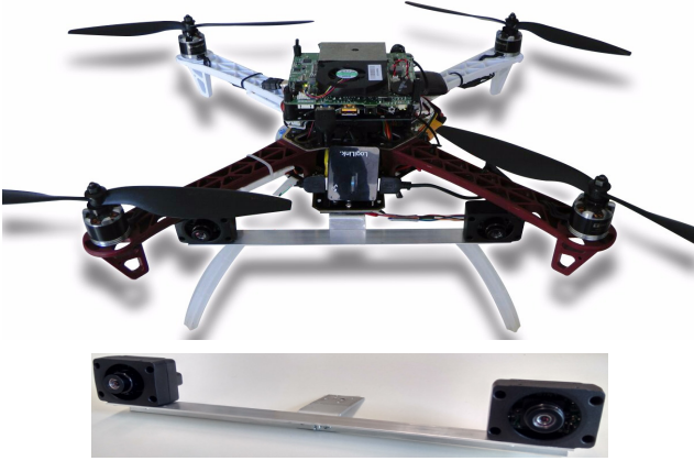
Fig. 7. Quadcopter used for our outdoor real experiments with the forward looking stereo camera.
