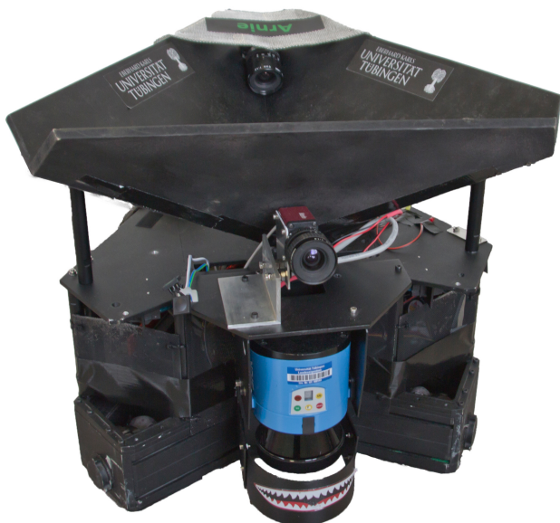
Fig. 1. Front view of one of our two robots with a hopper on top. Visible sensors: Allied Vision Marlin (center), PointGrey Firefly (top, inside the hopper), SICK LMS100 (bottom).
